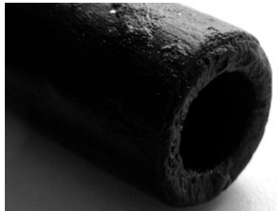
Fig. 21 The tube end of pipe T3 showing where the taper was removed.
