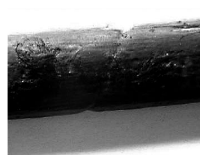
Fig. 18 The pressure indent around the surface of pipe T3.
