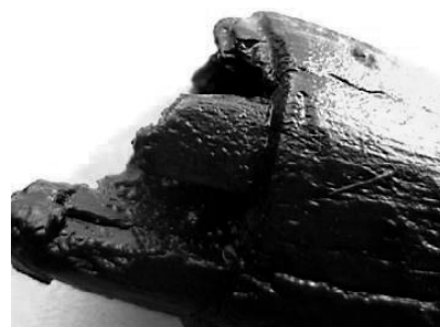
Fig. 10 The undercut at a pipe's tapered end.
