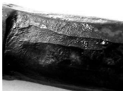
Fig. 12 Tool marks on the rebate at the obliquely-terminated end of a pipe.
