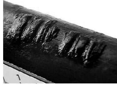
Fig. 20 Accretions on tube T1's outer walls.
