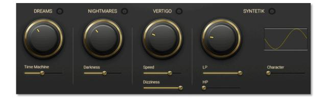
DREAMS | Hazy effect using chorus and delays. Main Knob: Chorus intensity. Time Machine: Chorus delay and feedback.
